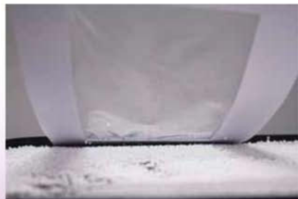
Polyethylene film with inclusion of Antistatic additive
