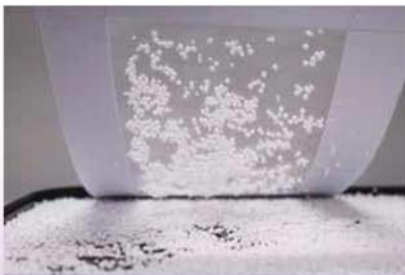
Polyethylene film without Antistatic additive
